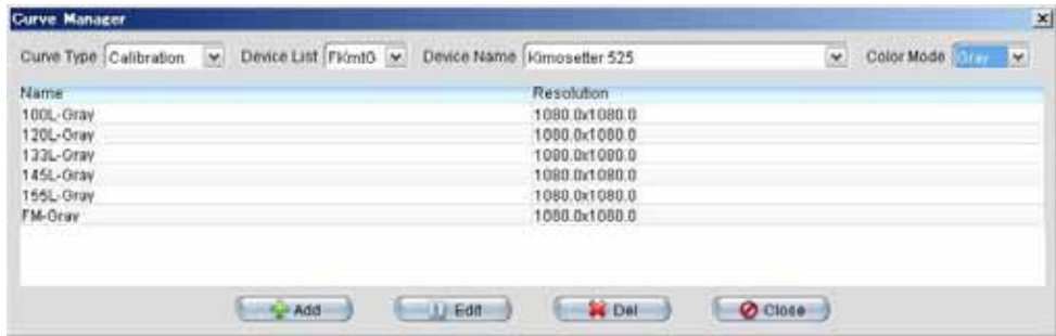
Fig. 2 Calibration curves for Gray displayed in curve manager. (All the curves except FM-Gray are in the CD supplied at the training course)
